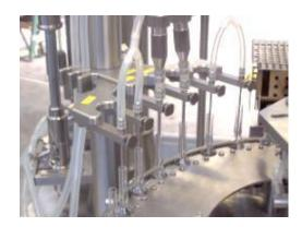
Objects are filled by mean of rotary piston pumps (accuracy better than  $\pm$  0.5%).
