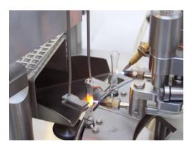
After the flame sealing station, the filled and sealed ampoules are gently pushed out of the transport star wheel by an exiting finger into the outfeed magazine.
