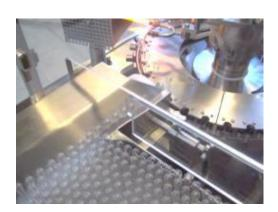
The inclined metal belt gently pushes the bunch of containers towards the infeed screw, which separates and transports them to the main star wheel. The transport star wheel hands gradually the containers over the machine through the opening station for ampoules (option), filling station (pre-gassing, gassing during filling and post-gassing are optionally available) and sealing station for ampoules or stoppering station for vials. Thus a careful object transport is ensured.
