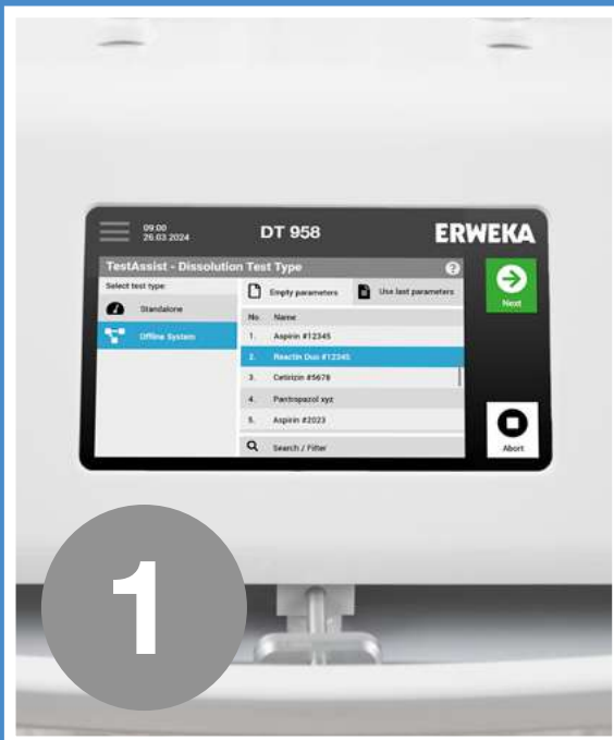
Step 1: Select your desired test type and click on a created method or empty parameters.
